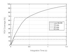
The FOV coverage of Livox Mid-360 and non-Livox LiDAR sensors using common mechanical scanning methods. The 16-line non-Livox LiDAR sensor has a vertical FOV of 30°, the 32-line non-Livox LiDAR sensor is 41°, and the 64-line non-Livox LiDAR sensor is 27°.
