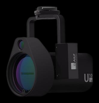
1.The U10 is a light-weight, high-sensitivity gas detector based on Tunable Diode Laser Absorption Spectroscopy (TDLAS), which enables rapid identification of methane from up to 100 m away, or at a concentration as low as 5ppm.m. Powered by DJI SkyPort, the U10 can be seamlessly integrated with DJI Matrice 200 Series V1 and V2 platforms.
