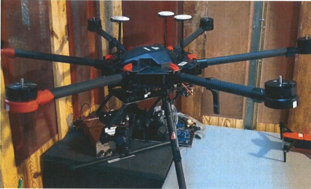
Figure 6. DJI Matrice 600 Pro within the RF-shielded chamber with propellers removed.
